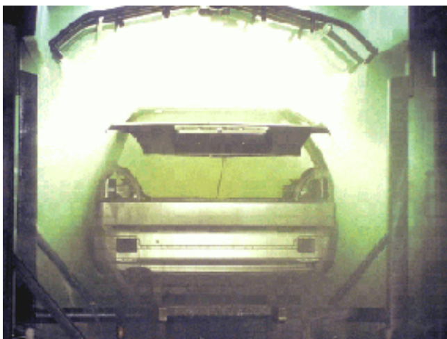
Figure 2.4: Automotive body undergoing spray pre-treatment [ACEA]
